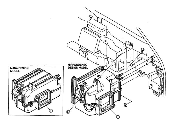
iii. Remove the outer box to expose the inner hose and hard lines. This consists of removing a few clips and a few screws. When the box shells come apart you'll have to pull the thermoswitch's sensor wire out of the core which is as simple as pulling it straight out.
