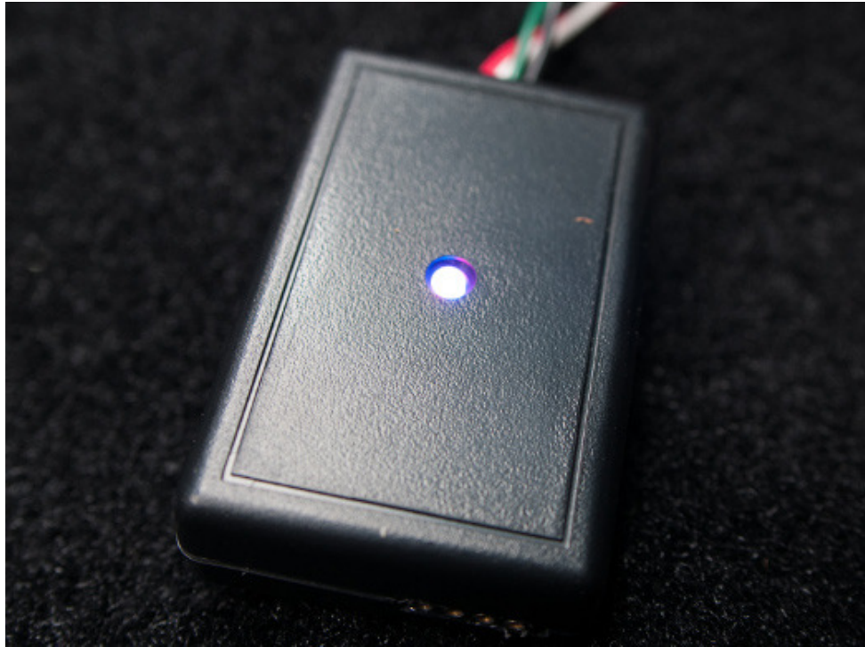
RPM switch with purple indicator light (car on and idling)
