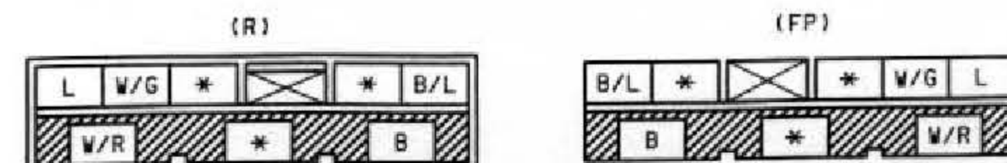
X-24 CONNECTOR BETWEEN REAR (R) & FUEL PUMP (FP)
