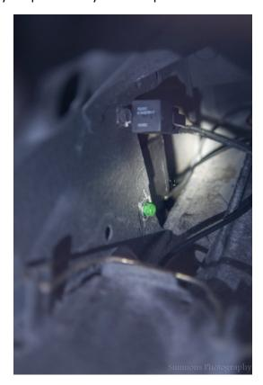
6. With the nut removed, you can reach in, grab the assembly, and gently push it back so that is retracts from the frame hole and the antenna mast surround drops out of the body hole. Maneuver the assembly and pull it out of the hatch access panel.
