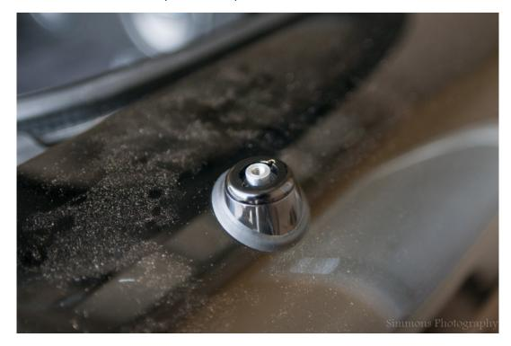
24. Push the assembly's stud through the mounting hole inside and loosely tighten up the inside nut. With everything loose but aligned, tighten the captive hat until it locks.
