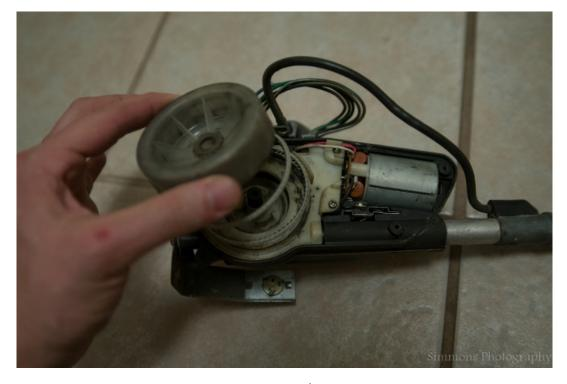
\*Note The flexible gearing for the antenna will coil / spill out. This is ok
