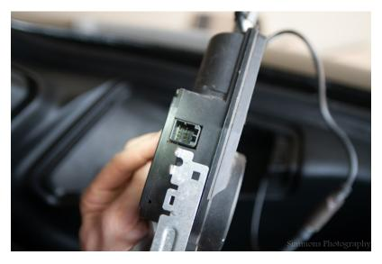
\*Note\* The retracting mast wiring <u>will not</u> be reconnected because without the mast you don't need the base to do anything except conduct signal from the antenna and that's a completely passive operation.
