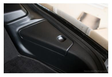
5. Look inside and spot the nut inside that bolts the antenna assembly to the body then work your arm and socket wrench inside to loosen and remove it. The antenna assembly has a stud that's pressed/welded to its frame, so it will just unscrew and it won't just fall out, but be careful that you don't accidentally push the antenna assembly too roughly because at this point with the captive hat and the nut removed, the assembly is loose and can potentially drop down in your rear quarter.
