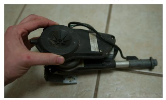
14. This is the goal. You want to get down to the point where the antenna outlet is stripped down where you can see the black plastic cup/liner inside the mast support
