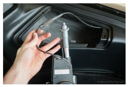
21. Maneuver the assembly into the access panel
