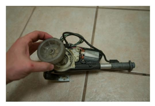
13. Now replace the lid to the antenna base unit and re-engage the 5 fastening screws
