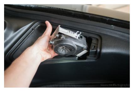
\*Note\* In the step above I had enough slack in my wiring to pull the assembly out before I unhooked the wiring, but all my wiring is aftermarket and I don't have the power wiring hooked up, so you 'may' have to do this while the antenna is still mounted before you can pull it out.
