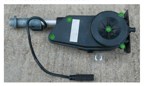
10. Remove the top cover and pull the antenna's gear cover off
