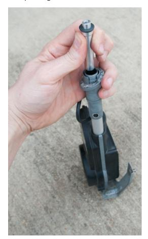
16. At this point you'll feel resistance when pushing the adapter in. This is where you encounter the press fit. It's a lite interference fit so you can press it in by hand but if its uncomfortable to press / tighter than expected you can use something like a block of wood to help spread the point of contact while pressing it in.
