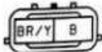
J4-07 – Rear Hatch Lock Key Cylinder Switch (R) Page 90 J4-07 REAR HATCH LOCK KEY CYLINDER SWITCH (R)
